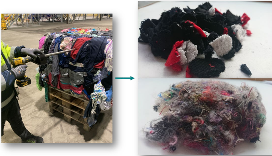
Figure 2: Demonstration of the sampling method used in the Siptex project, in which drill samples are taken using a hay sampler (left picture) and an example of the shredded and homogenized samples that were sent for analysis (right pictures).
