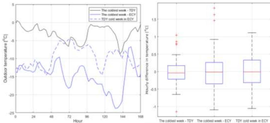
Figure 13. Comparing the coldest week in a typical year (TDY), an extreme cold year (ECY) and the situation of the TDY cold week in ECY over 2040-2069 (representing 2050). The average weekly temperature for the cases are -3.1, -14.8 and -9.6°C, respectively, with the standard deviations of 2.1, 3.8 and 2.9°C.
