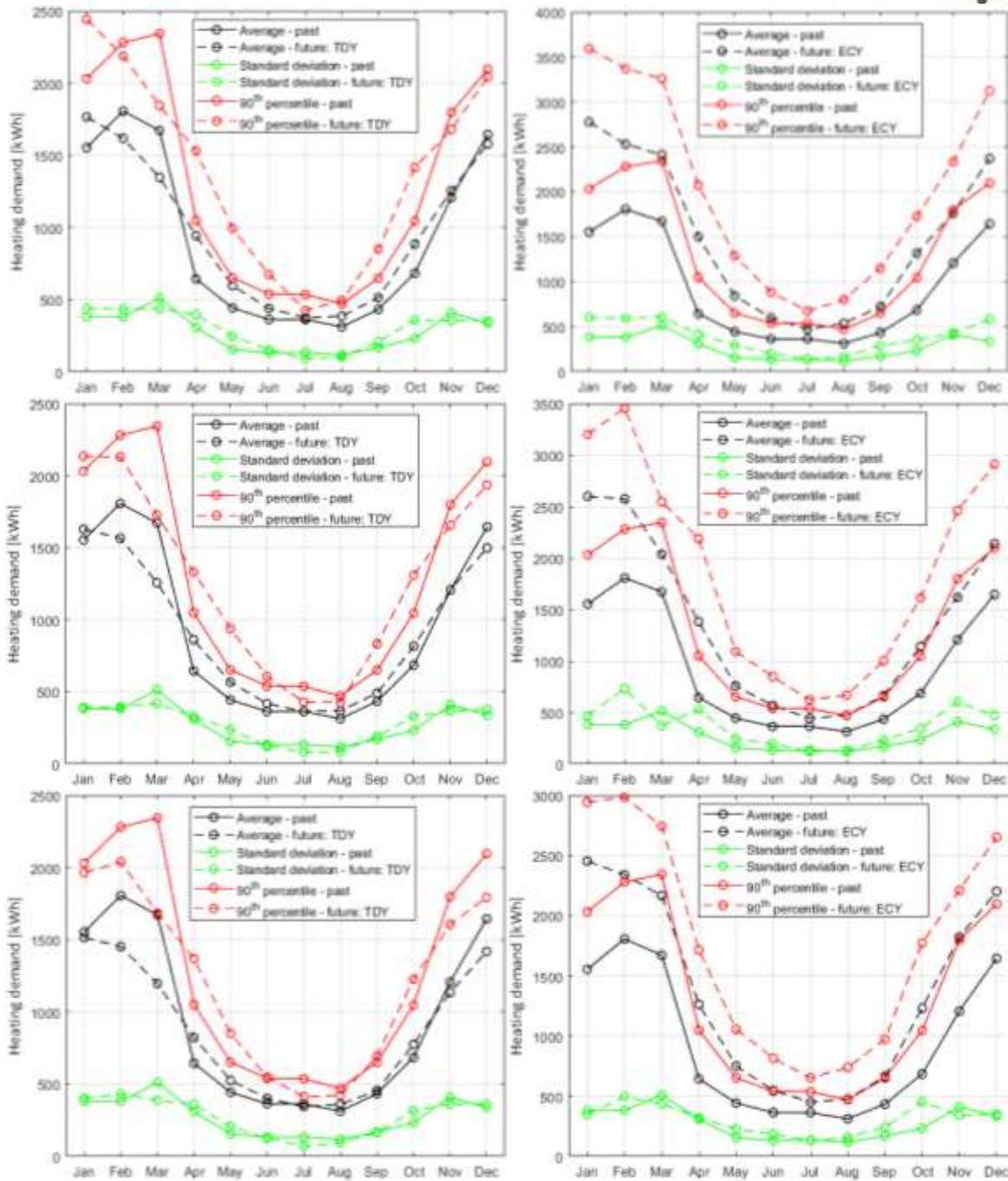
Figure 16. Comparing monthly average, standard deviation and 90<sup>th</sup> percentile values of heating demand for TDY (left) and ECY (right), in Maria Laach during 2010-2039 (top), 2040-2069 (middle) and 2070-2099 (bottom).
