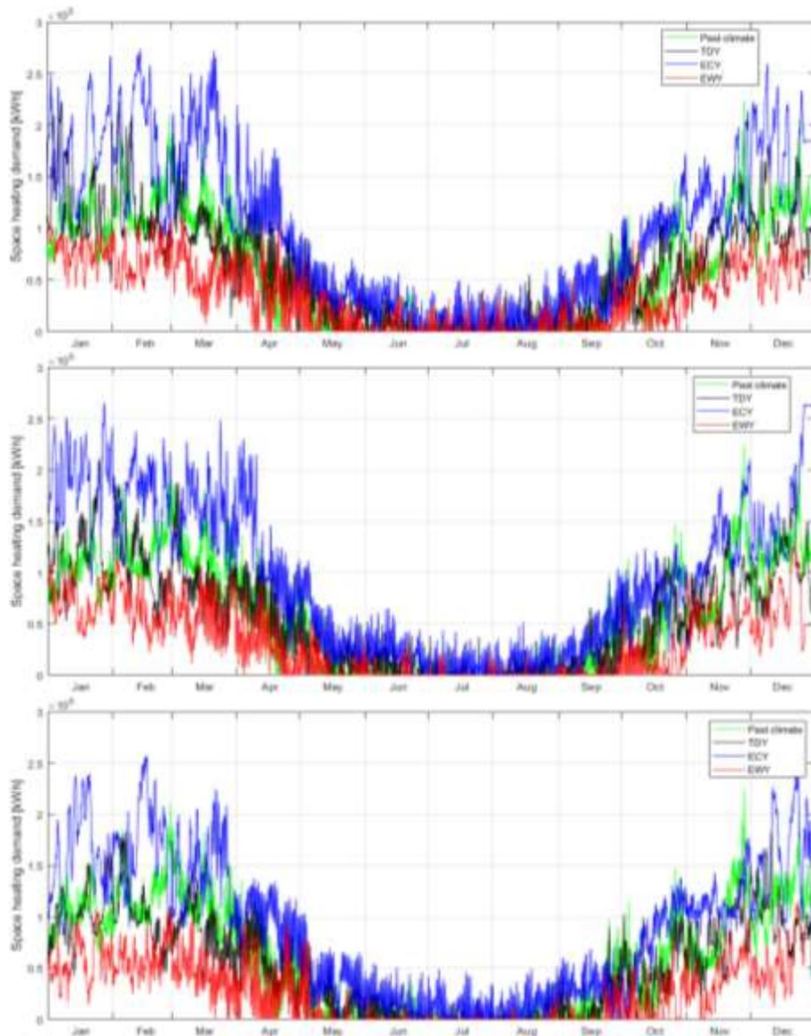
Figure 5. The hourly profiles of space heating demand in Eskilstuna for three time periods, considering typical (TDY), extreme cold (RCY) and extreme warm (EWW) years.
