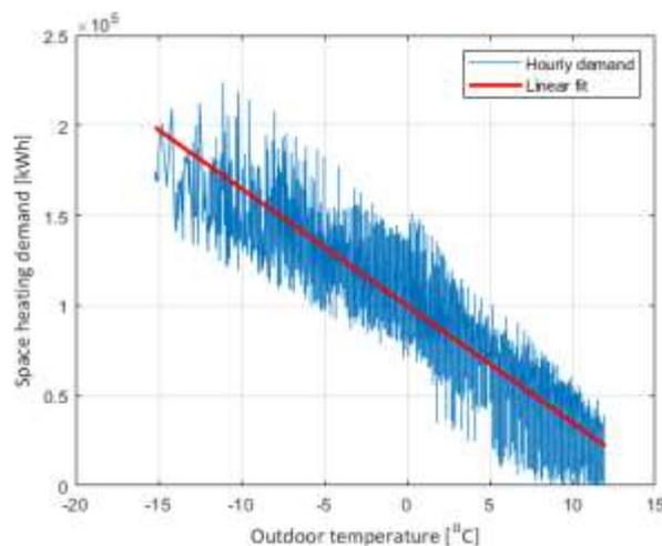
Figure 2. Sorted heating demand for Eskilstuna and the linear fit line, used as the estimation function to generate the future energy demand during three time periods.
