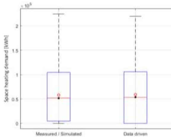
Figure 3. Comparing the distribution of the measured/simulated space heating demand in Eskilstuna with the estimated demand using the linear regression model (data driven). The red squares represent the average values and black dots the calculated standard deviations.
