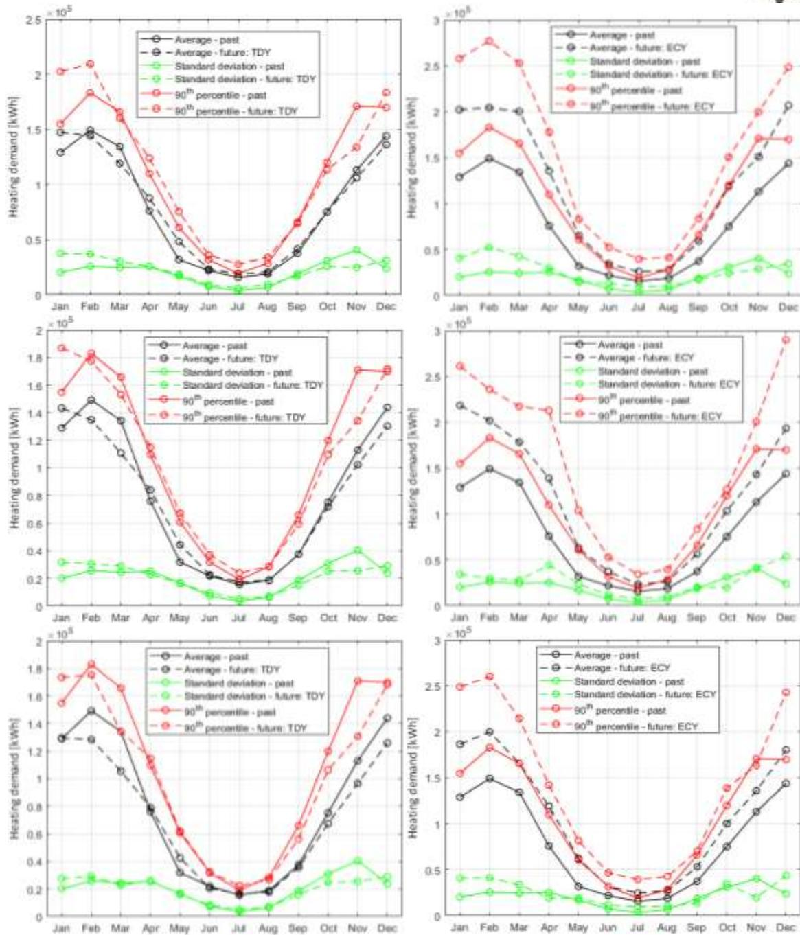
Figure 14. Comparing monthly average, standard deviation and 90<sup>th</sup> percentile values of heating demand for TDY (left) and ECY (right), in Eskilstuna during 2010-2039 (top), 2040-2069 (middle) and 2070-2099 (bottom).
