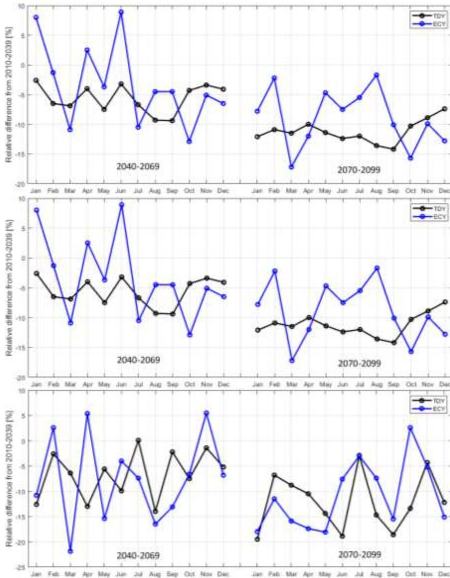
Figure 17. Relative difference in the monthly average (top), standard deviation (middle) and 90<sup>th</sup> percentile (bottom) heating demand in two periods compared to 2010-2039 in Maria Laach.
