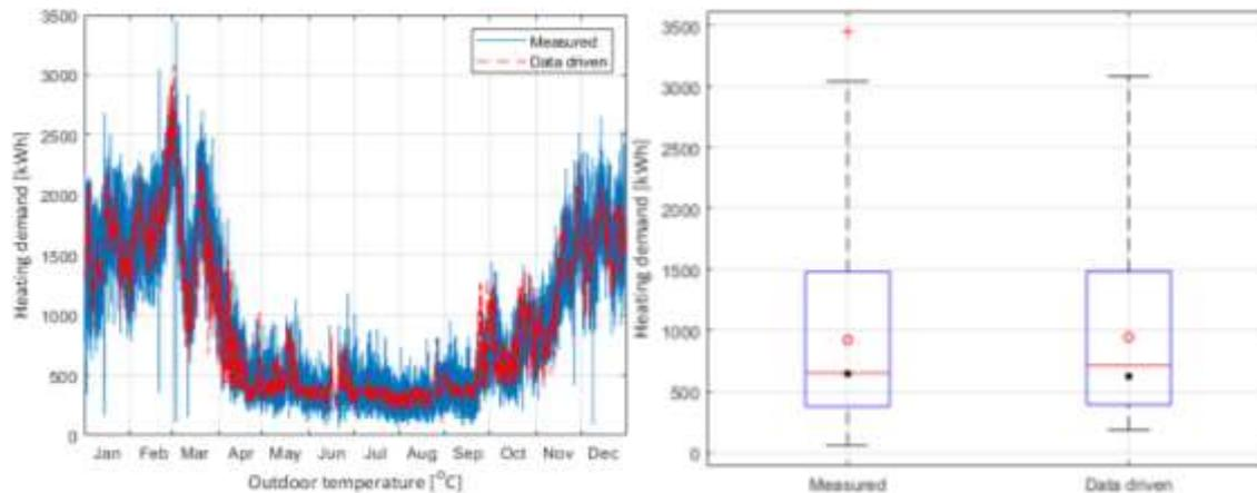
Figure 4. Comparing the hourly profile and annual distribution of the measured and estimated (data driven) heating demand in Maria Laach. In the boxplots, the red circles mark the average values and black dots the calculated standard deviations.
