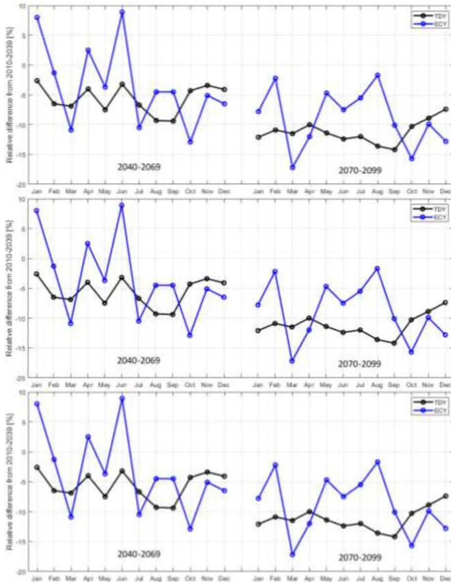
Figure 15. Relative difference in the monthly average (top), standard deviation (middle) and 90<sup>th</sup> percentile (bottom) heating demand in two periods compared to 2010-2039 in Eskilstuna.
