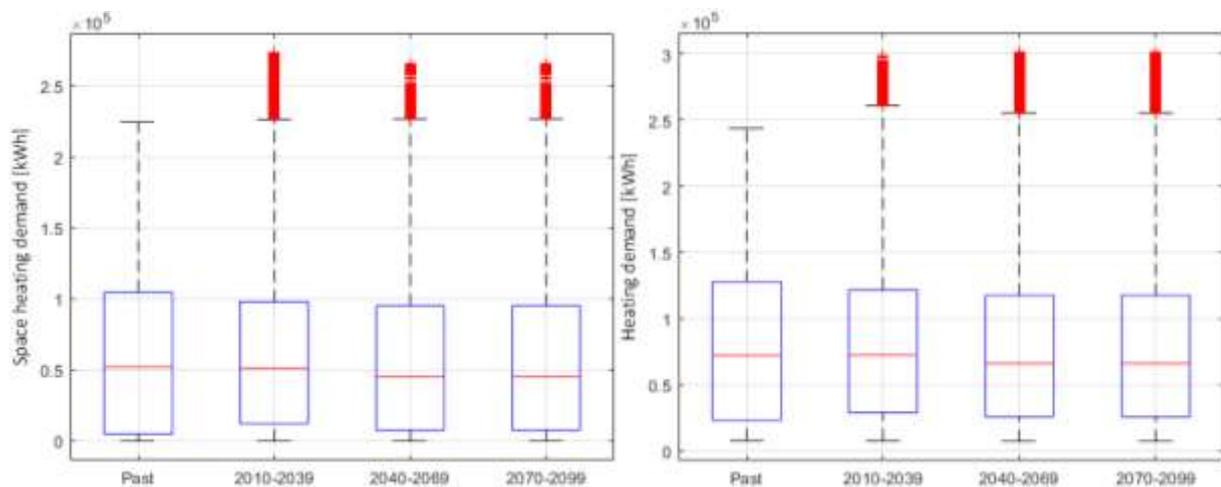
Figure 6. Comparing the distribution of the (left) space heating demand and (right) total heating demand (space and hot water heating demand) over past climate (2018) and three future periods in Eskilstuna.
