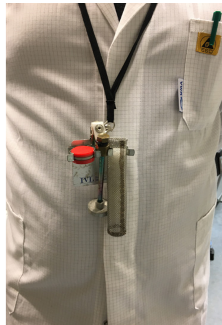
Set of samplers for measuring several different air pollutants. Nitrogen dioxide (red button), sulfur dioxide (blue button), ozone (white button), volatile organic compounds (steel tube), polycyclic aromatic hydrocarbons (foam in protective net) and formaldehyde (white tube in the middle). The seal on the steel tube is removed to start the measurement.
