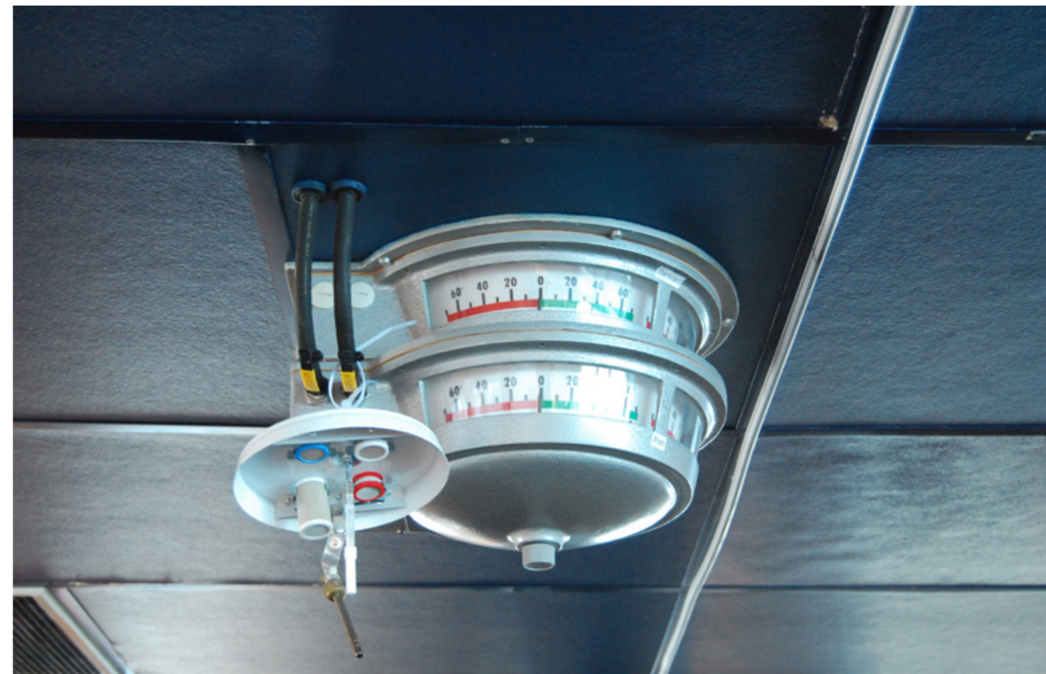
Set of samplers for measuring several different air pollutants. Nitrogen dioxide (red button), sulfur dioxide (blue button), ozone (white button), volatile organic compounds (steel tube), polycyclic aromatic hydrocarbons (foam in protective net) and formaldehyde (white tube in the middle). The seal on the steel tube is removed to start the measurement.
